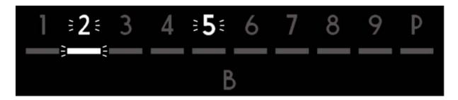
The cooktop is not properly connected to the electrical network. Check the power connection.
